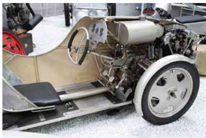
Neander Fahrmaschine 1, 1937, HD Knucklehead motor
